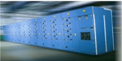
MCC are offered upto 1600 A operational current at 40 degree Celsius ambient Temperature in single and double front design for 50 kA short Circuit Withstand Capacity and IP: 52 degree of Protection. Form IV of separation as per IS: 8623 is maintained. Types of starters include Automatic Star Delta, Direct On-line, Soft Starters, Variable Frequency Drives, Stator Rotor Starters and AutoTransformer Starters.
