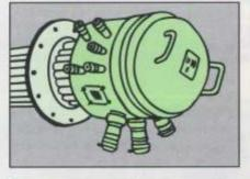
The dimension of the box determines the maximum number of heating elements of dia. 16 (R16) and the bundle diameter (0). See Table below.
