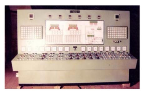
Custom-made control desks, with fiber glass or acrylic mimic diagrams, completely equipped with annunciation equipment, are designed and manufactured by us for all types of Process Control Industries.
